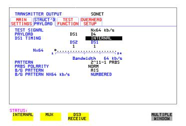
5 Choosing DS1 gives the timing choice shown above. Select INTERNAL to time the DS1 signal from the internal clock in the OmniBER transmitter; select MUX to time the DS1 signal from the signal applied to the OmniBER via the mux/insert
